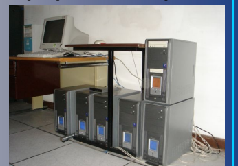
Figure 6 THOR: a 6 AMD 64 PC cluster with main characteristics: chipset ASUS ASN-E, 1Gb RAM, 129 Gb disk space, graphical ATI Radeon 65 Mb card
