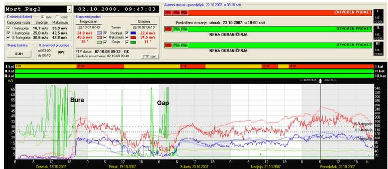
Example of the well predicted Bura for Station Most Pag 2. Red lines represents wind gust, blue mean wind speed and green wind direction. Light lines represent Aladin 2km dynamical adaptation forecast, heavy lines represents measurements.
