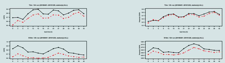
CRPS of ECEPS (black full line) and GLAMEPS (red dashed line) for bias corrected T2m (top) and S10m (bottom) (run=12h).
