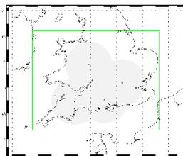
Figure 6. a) NDP domain showing radars producing Doppler radial winds Jan 2011. From left to right - Cobbacombe, Clee Hill, Dean Hill, Chenies. b) Below: NDP domain (green) nested in UK4 and UKV domains.
