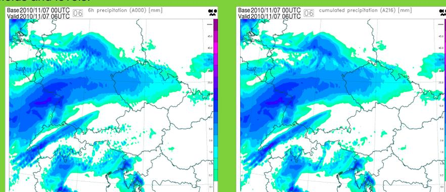
The 6 hour precipitation with operational SLHD settings (left). Short scale noise clearly visible above parts of Germany and Czech Republic was significantly reduced with retuned spectral part of SLHD (right).
