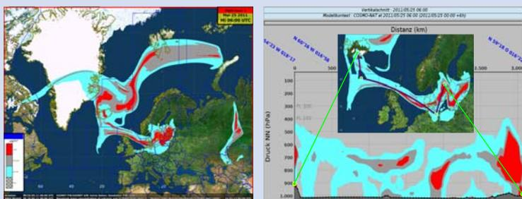
Maximum mass concentration of volcanic ash in the layer between the surface and flight level 200 (approx. 6100 m above ground).
