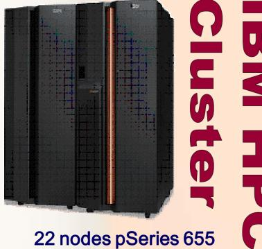
22 nodes pSeries 655 8-way 1.7GHz Power 4+ 16 GB memory two-link switch interface
