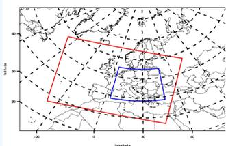
Figure 1: ALADIN-LAEF domain (18 km horizontal resolution) is depicted in red (large box). The verification domain, which covers Central Europe, is given in blue (smaller box).
