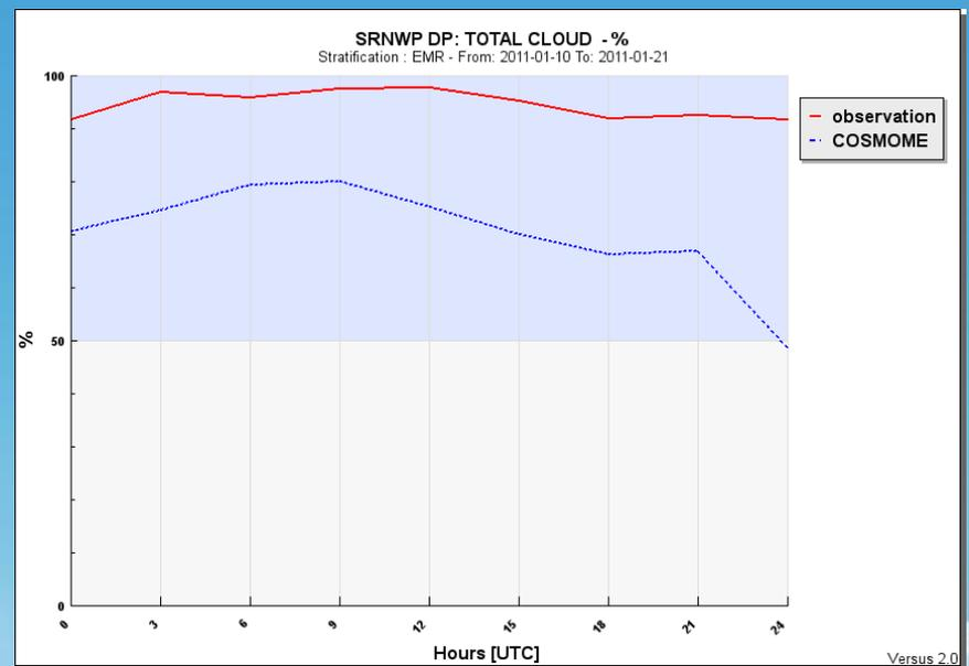
Model predicted wrong values for LW balance but also a completely wrong TCC (much less than reality)
