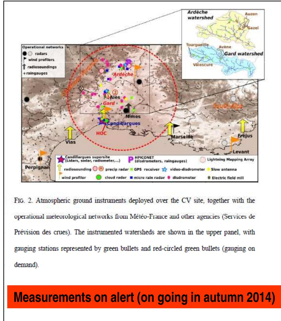
FIG. 2. Atmospheric ground instruments deployed over the CV site, together with the operational meteorological networks from Météo-France and other agencies (Services de Prévision des crues). The instrumented watersheds are shown in the upper panel, with gauging stations represented by green bullets and red-circled green bullets (gauging on demand).
