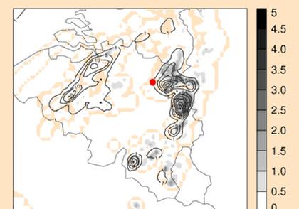
FIG 1: Sub-grid scale downdraft mass flux (units: kg/m²s) as forecasted by Alaro with the unsaturated downdraft scheme for 1700 UTC, 18 August 2011. Rain rate is shown by black contours (lines for 1, 5, 10, 20, 30, 40 and 50 mm/h). The location of the Pukkelpop festival is shown with a red dot. The downburst at the Pukkelpop festival occurred at 1615 UTC.
