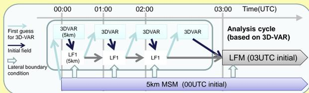
Fig. 2: A schematic diagram of the data assimilation system which provides an initial field for LFM.
