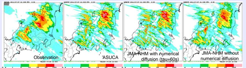
Fig. 6: Sensitivity to numerical diffusion. As the numerical diffusion is stronger, convective cells are shifted to more downstream side, i.e. convective initiation is delayed compared to smaller diffusion case. Convective initiation is affected by unresolved small modes. Unresolved part should be parameterized.
