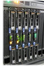
As a front-end to the HPC machine, an high-availability virtualization system will be used, the IBM Blade Center. Each node is a Xeon X5650 with 6 cores at 2,67 GHz; 36 GB of RAM is also available. Linux (Ubuntu) and Windows will be used as OS. The system is also suitable for visualization, pre- and post-processing.
