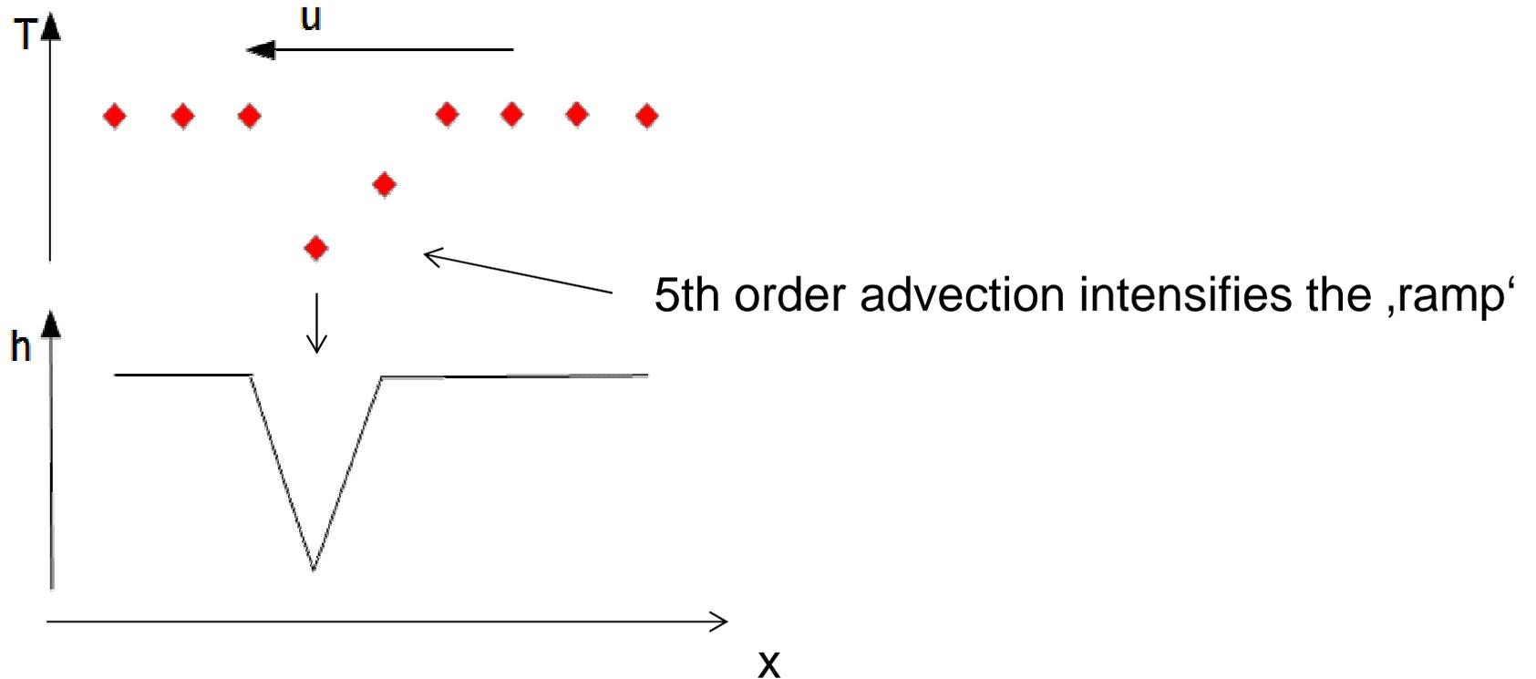
Linear advection equation (1-dim.)  $\frac{\partial q}{\partial t} + u \frac{\partial q}{\partial x} = 0$  discretized:  $\frac{q_j^{n+1} - q_j^n}{\Delta t} = f_j(q^n)$
