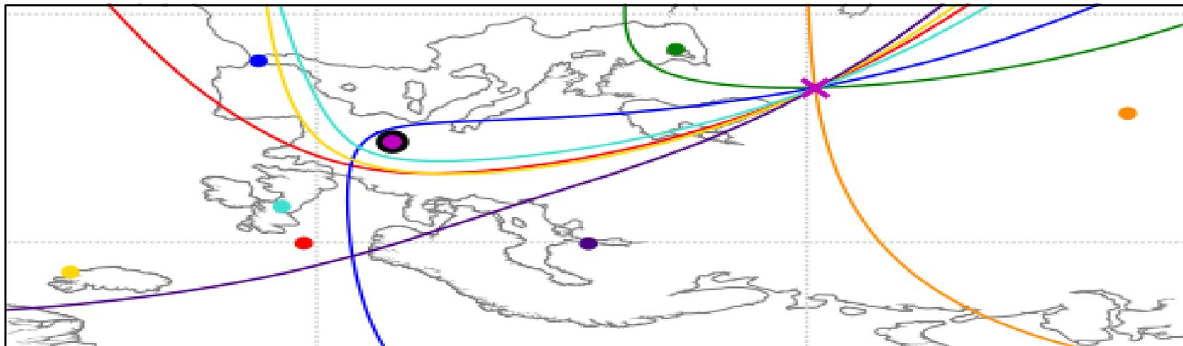
Hyperbola plot - the potential locations of the lightning source from every pair of stations, the intersection of all the hyperbolae is the lightning location.
