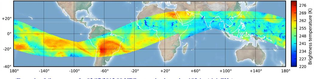
(Example of 6h coverage for 02/07/2012 00 UTC network; channel at 183.1 +/-1.1 GHz)
