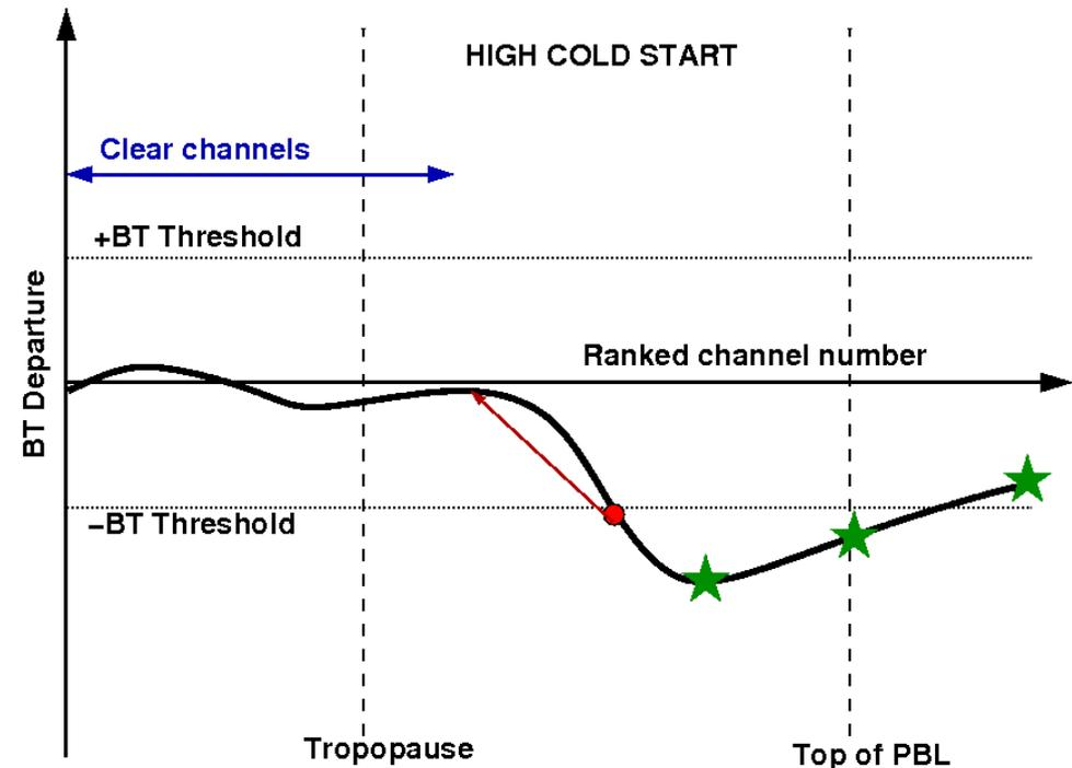
*cloud detection algorithm as used for assimilation of AIRS, IASI and CrIS data by McNally and Watts (2003)*
