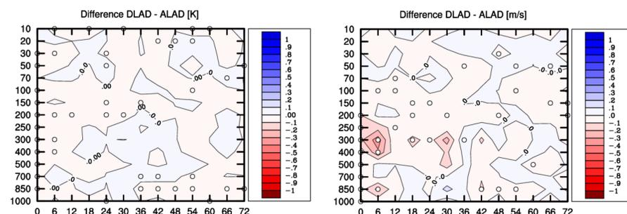
Figure 2: RMSE differences of temperature (left) and wind speed (right) for period of 11 May – 20 Jun 2017 12UTC. Red areas denote better performance of optimized aircraft data assimilation with respect to operational runs. The white circles point that RMSE difference is better/worse with significance 95% two-side confidence interval.
