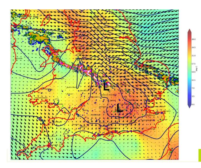
WOW surface analysis at **1600** UTC 27 May 2018 showing surface temperatures (shading), wind vectors (arrows) and MSLP (dark blue contours, contour interval 0.5 hPa) with composite radar rainfall rate overlaid.
