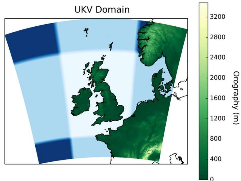
The UKV uses a rectangular grid in rotated lat-lon coordinates with variable spacing. The sea is coloured according to grid box area (with 4x4km boxes dark blue)
