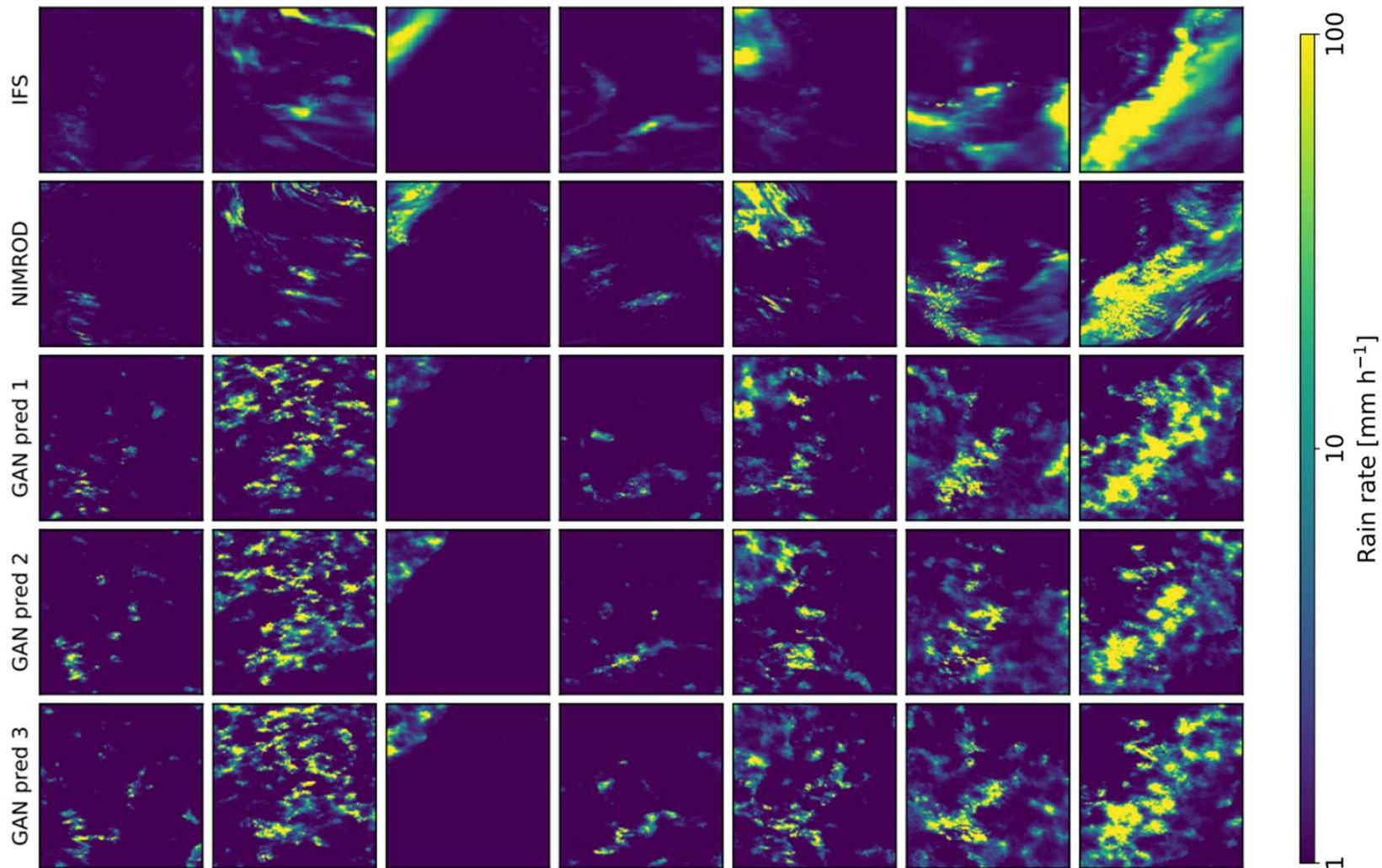
Map IFS model data at  $\sim 10$  km resolution to NIMROD precipitation observations at  $\sim 1$  km resolution
