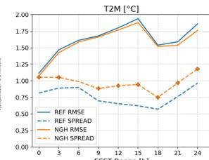
Fig. 3. The RMSE of the ensemble mean (solid) and spread (dashed) of reference experiment (blue) and NPP (orange) for 2-m temperature averaged over 62 days. Forecast ranges with statistically significant difference are highlighted using markers.
