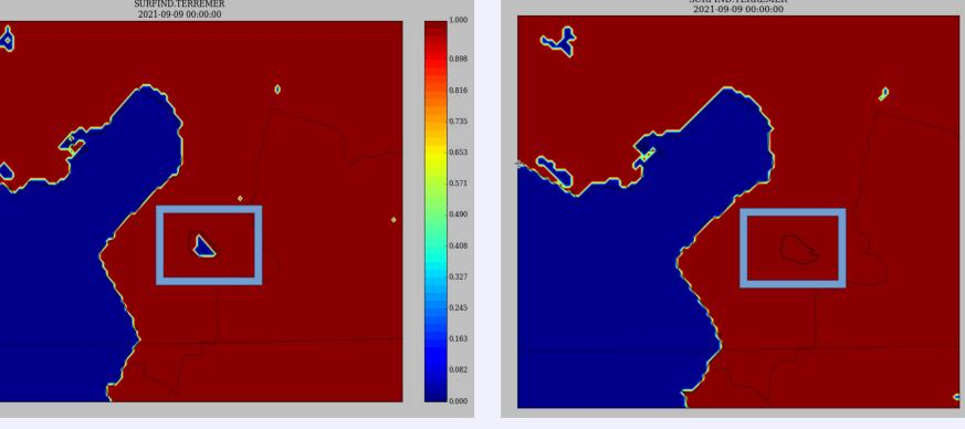
The removal of the lake (shown in blue rectangle) which does not exist in real, in AROME Turkey domain after using ecoclimap 2<sup>nd</sup> generation.
