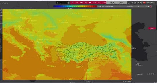
Representation of A-LAEF products on TSMS interactive web page (10m wind probability forecast for threshold between 15-25 knot and hourly total precipitation probability forecast for threshold between 1-52 mm on top. Spaghetti plot of geopotentiel height at 500 hPa and ensemble mean plot of 2 meter temperature at bottom).
