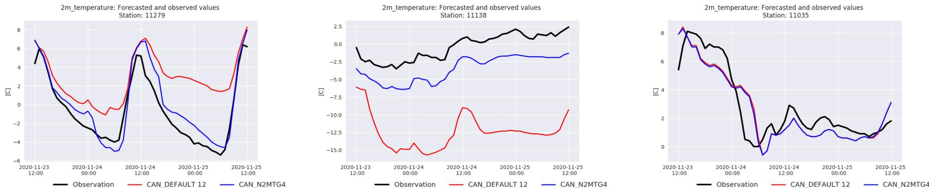
forecasts and the observed 2m temperature for a station located in a valley (left), on a mountain top (middle) and in the flatlands (right) for 23<sup>rd</sup> November 2020, 12 UTC run.
