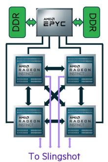
2560 nodes with 4 x MI250X + 1 x AMD Trento processor, 512 GB host memory and 512 GB device memory (HBM<sub>2</sub>) 4 x 200 Gbit/s NIC Infinity Fabric
