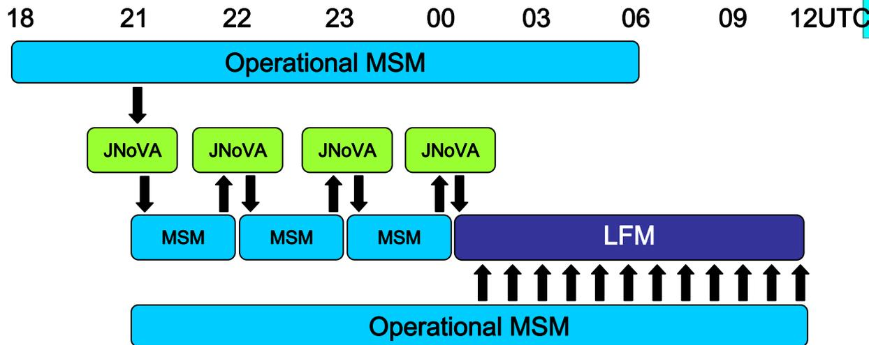
Schematic diagram of the analysis forecast system of LFM
