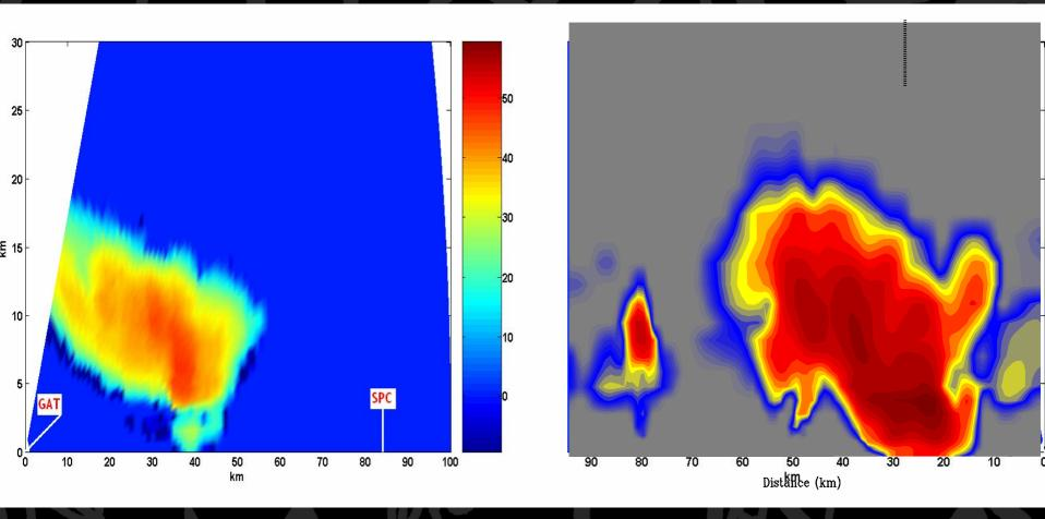
Vertical section (RHI) of copolar reflectivity  $Z_{HH}$  with respect to the line of sight between the two C-band radar systems on May 20, 2003 at 17:30 UTC simulated by means of the COSMO-LAMI/RSM-POL chain nested on the SETTING-3 COSMO-LAMI run *("light graupel")*. On the right, a RHI derived from MM5 reflectivity compution model nested on SETTING-3 MM5 run (at 18.00)
