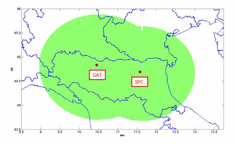
Gattatico (GAT, left) and S. Pietro Capofiume (SPC, right) are two C-band polarimetric radars, with a maximum range of about 100 km owned by ARPA-SMR Emilia-Romagna. The distance between the two is about 90 km.
