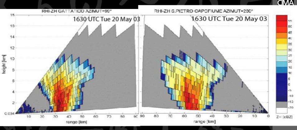
Vertical section (RHI) of copolar reflectivity  $Z_{HH}$  with respect to the line of sight between the two C-band radar systems in Italy on May 20, 2003 at 16:30.
