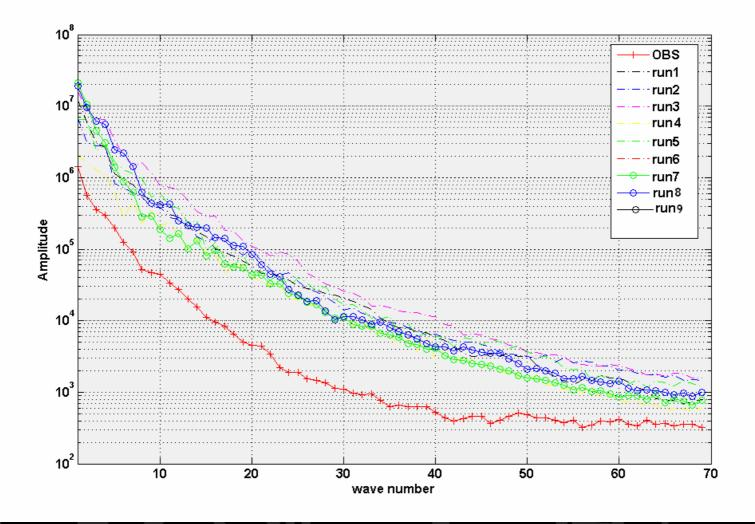
Mean spectra for both observed SPC water content (in red) and simulated (other colors)
