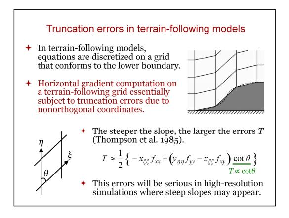
Horizontal gradient computation on a terrain-following grid essentially subject to truncation errors, because the horizontal gradient at this cell, for example, is calculated from the values at these neighboring cells, and the deviation from the exact horizontal direction causes the errors described as this. The steeper the slope, the larger the deviation, and the larger the errors. You can get details from this book, Thompson et al..
