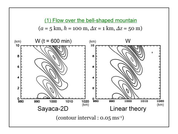
This is the result in the case of the bell-shaped mountain after attainment of quasisteady state. The horizontal and vertical grid intervals that we used are 1 km and 50 m, respectively. This shows the vertical velocity field calculated by our model, and this shows that by the linear theory. The vertical velocity calculated by the model agrees well with that in the analytical solution.
