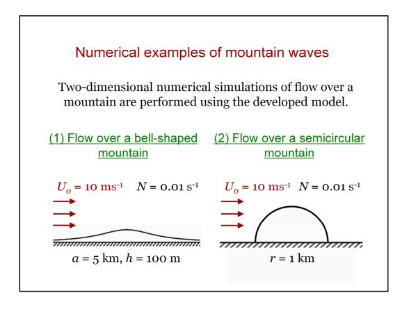
Now, let me talk about results. We performed two-dimensional numerical simulations of flow over a mountain using the developed model. Here, two mountains are used. One is a low bell-shaped mountain with gentle slopes. The other is a semicircular mountain which has very steep slopes at the foot. The constant horizontal velocity and Brunt-Vaisala frequency are specified for both cases.
