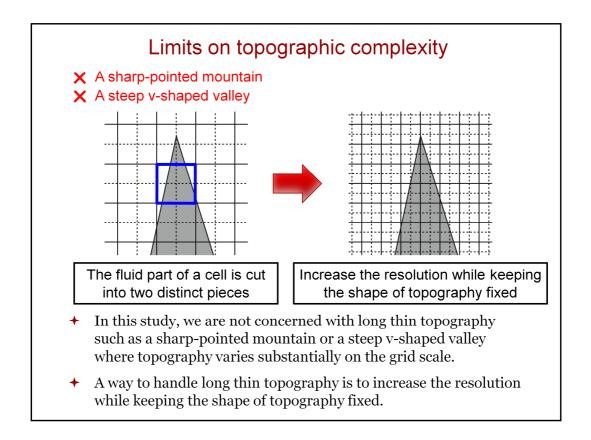
In this study, we are not concerned with long thin topography such as a sharp-pointed mountain or a steep v-shaped valley. For example, this sharp-pointed mountain cuts a cell into two distinct pieces, and our method is not applicable to this situation. A way to handle long thin topography is to increase the resolution while keeping the shape of topography fixed like this to avoid topographic changes on the grid scale.
