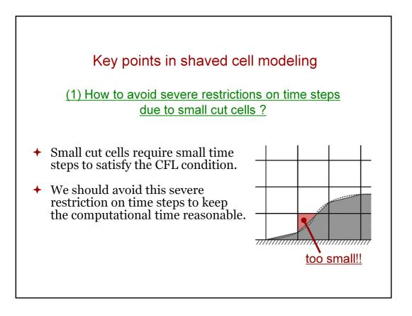
Now, there are two key points in shaved cell modeling. The first point is how to avoid severe restrictions on time steps due to small cut cells. Small cells cut by topography, such as this cell, require small time steps to satisfy the CFL condition. To keep the computational time reasonable, we should avoid this severe restriction on time steps in some way.
