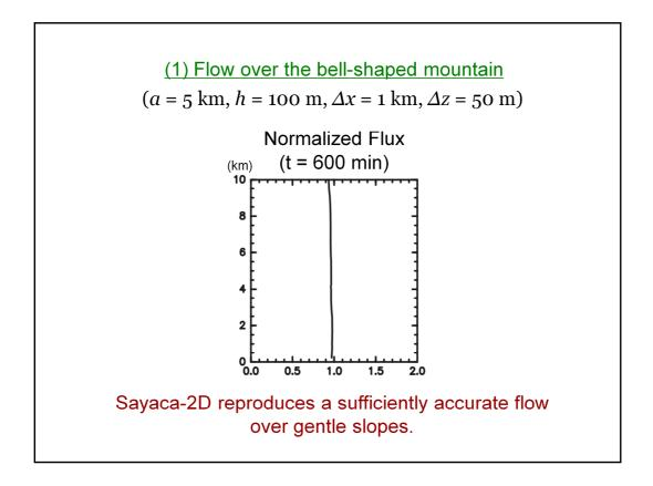
This is the momentum flux in our model normalized by that in the linear theory. It is nearly uniform from near the surface to 10 km, thus the momentum flux in model agrees well with that in the linear theory. Thus we conclude that our model reproduces a sufficiently accurate flow over gentle slopes.
