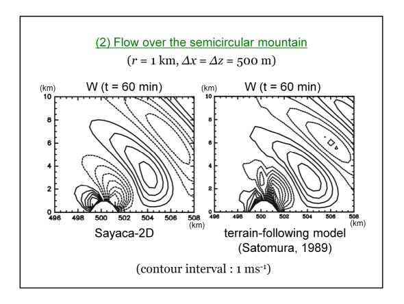
Next, this is the result in the case of the semicircular mountain after attainment of quasi-steady state. Here, both the horizontal and vertical grid intervals are 500 m.
