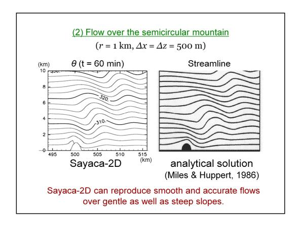
Finally, this shows the potential temperature field in our model, and this shows the stream lines of the analytical solution given by Miles & Huppert. They are similar to each other and it shows that our model reproduces an accurate flow over the semicircular mountain. Therefore, we conclude that our model can reproduce smooth and accurate flows over gentle as well as steep slopes, thus it is appropriate and sufficiently accurate for simulations of flow over complex terrain.
