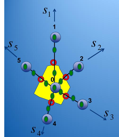
The scheme defined above is conserving, if the point fluxes defined above for points 0 and 1 etc compensate. This is achieved by defining the derivatives by collocation points obtained by interpolation or Galerkin methods.
