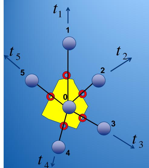
$t_1$ : directional parameter for line 0,1 etc  $f_1$ : point flux for point on line 0,1 etc  $\rho_1$ : density derivative for point 0 etc  $\mathcal{W}_1$ : weight to be defined for the point flux  $\frac{\delta f_i}{\delta t}$ : directional derivative
