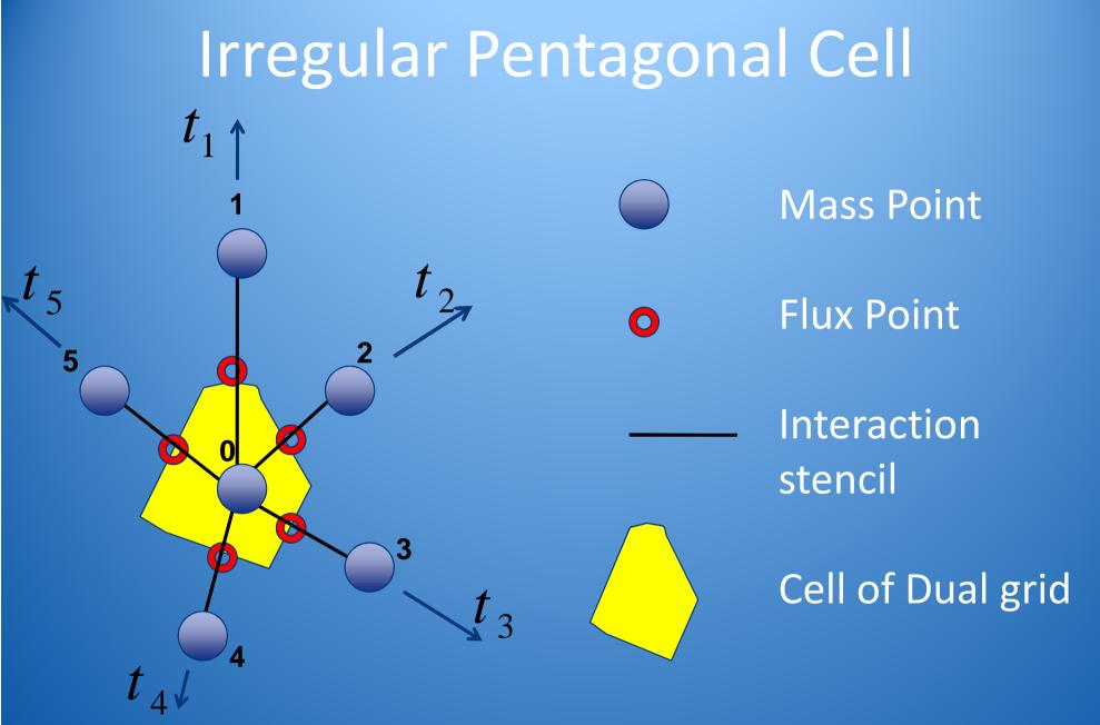
The grid is called quasi regular, if stencil lines cut the sides of the dual cell in half
