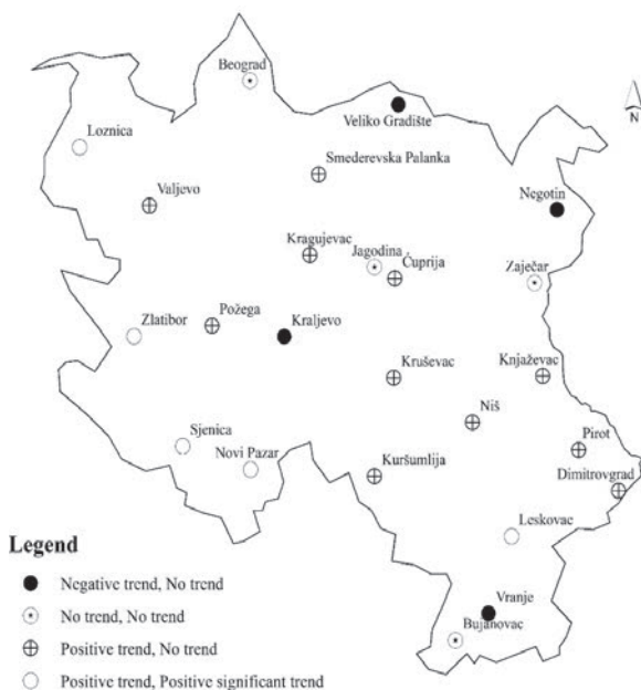
Fig. 3. Cartographic presentation of the obtained results of the linear equation and the Mann-Kendall trend test, respectively, for the total annual amount of precipitation in Central Serbia for the time period from 1949 to 2018.
